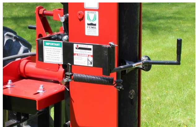
Drive Ram and Safety Arm with fence post.
