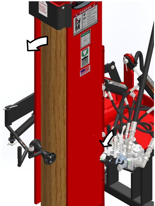
Tilt top of Drive Ram away from tractor/skid loader pull middle lever toward operator.
