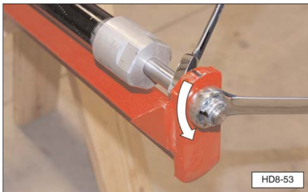
Loosen Lock Nut (C4) 1/2 Turn After Tightening.
