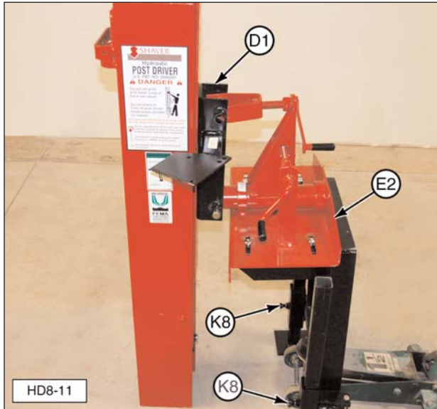
(D1) Short Channel Bracket. (E2) Base Plate. (K8) Stabilizer Leg Lock Bolts.
