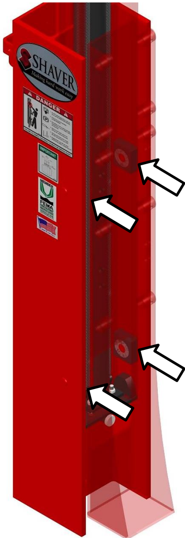
Guide Block/Roller locations (arrows) on Driver (HD-10 shown with transparent Main Carriage).
