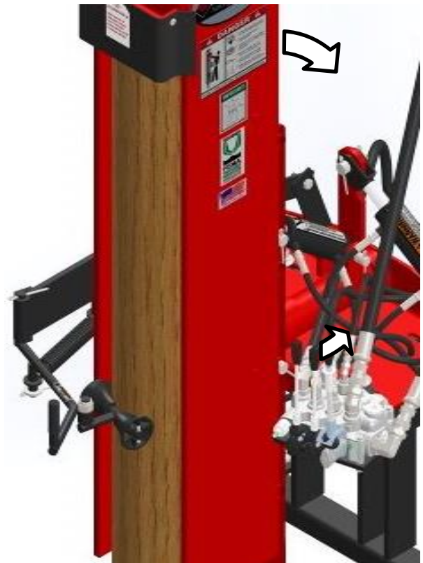
Tilt top of Drive Ram toward tractor/skid loader push middle lever away from operator.
