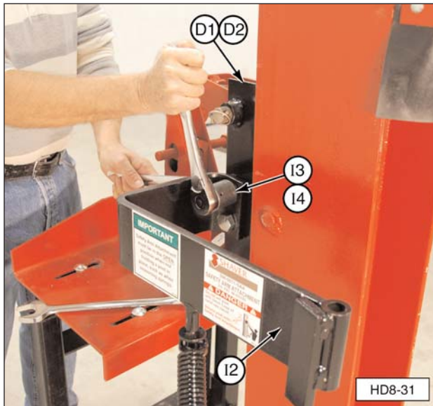
(D1) Manual Channel Bracket. (D2) Hydraulic Channel Bracket (not shown). (I2) Safety Arm Frame. (I3) Frame Mounting Bolt. (I4) Self Locking Nut.
