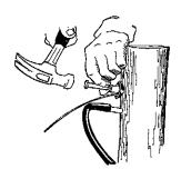
\*Cut the INSULTUBE into suitable (generous) lengths, load it with SPIDER Wire allowing at least 1" at each end to take the power around to each plug. Make sure the insultube is positioned to allow water to run out of the ends.
