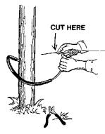
\* Hold the G-Spring against the post while pulling up the wire with the other hand to estimate a suitable point to cut it (pull the wire to about 20 pound tension and cut about one inch past the tip of the "G").
