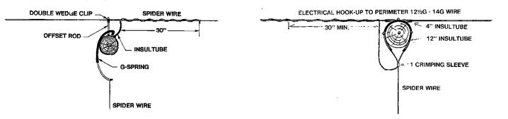
**SPIDER "GATES":** The Spider G-Spring offers access in many ways. It can be used to form a somewhat conventional gate by incorporating a very short span (60' or less) of Spider fence as a "gate span", or, costs can be saved by incorporating an "integral gate" in one of the ways shown below.G-Spring gates are not seen as a total substitute for all gate situations, such as main thoroughfares, where a more conventional gate may be required.
