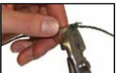
5. Fold other end over the first crimp, overlapping both sections. Crimp again so the twine is secure.
