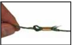
6. With scissors, trim excess twine for a clean repair.
