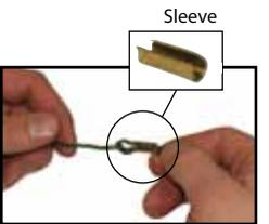
4. With a pair of pliers crimp one end of the sleeve over both pieces of twine.
