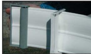
3. Insert (now properly shaped) end of rail into remaining buckle slot and press flat against buckle. With sufficient force, flatten assembly by pulling up on end of buckle and down on rail.
